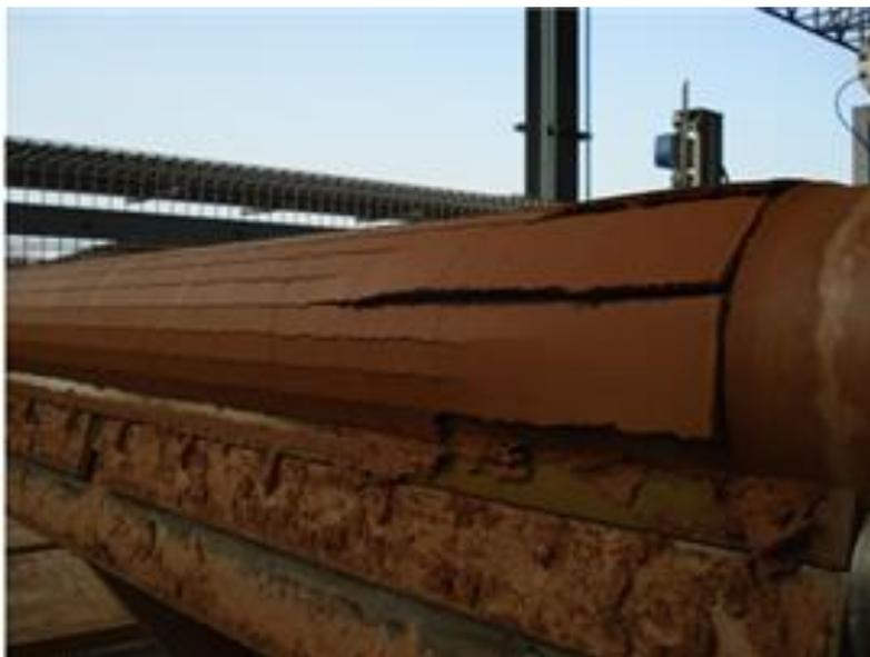
**Figure 2: Sample of IP coming off of belt filter (South America)**
