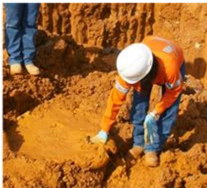
**Figure 6: Stockpiled IP shows stable vertical cut and vibration-induced liquefied bottom**
