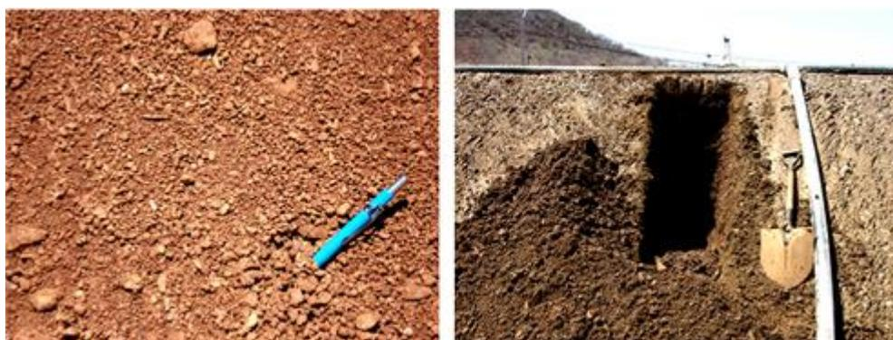
**Figure 1: Sample of fresh agglomerated ore (left) and ripios from pilot heap (Piaui mine, Brazil)**
